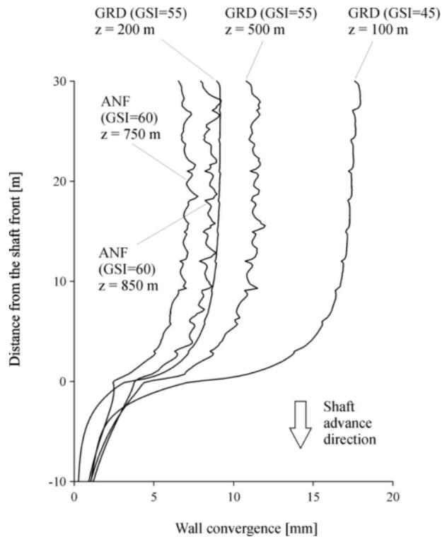
Figure 8. Longitudinal displacement profiles obtained from Phase2 axi-symmetric models for the five different conditions of shaft depth and geotechnical units expected to be encountered during excavation.
