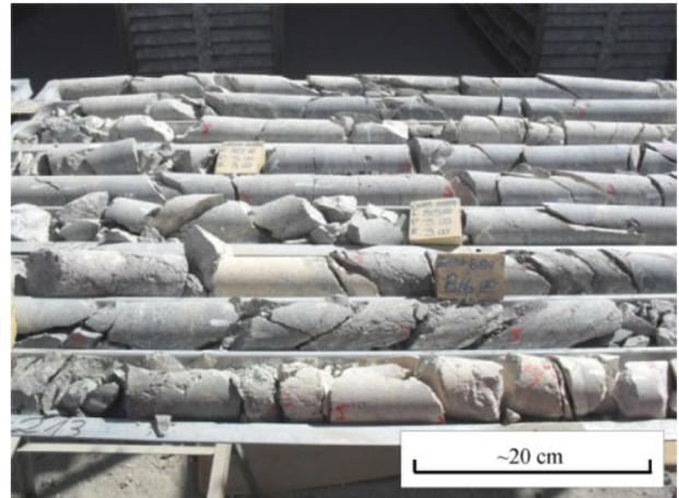
Figure 3. Core showing the Structurally Lixiviated unit (LXE) at depths 814-to-818 meters as recovered from perforation CHDD8184 – see Figure 2.
