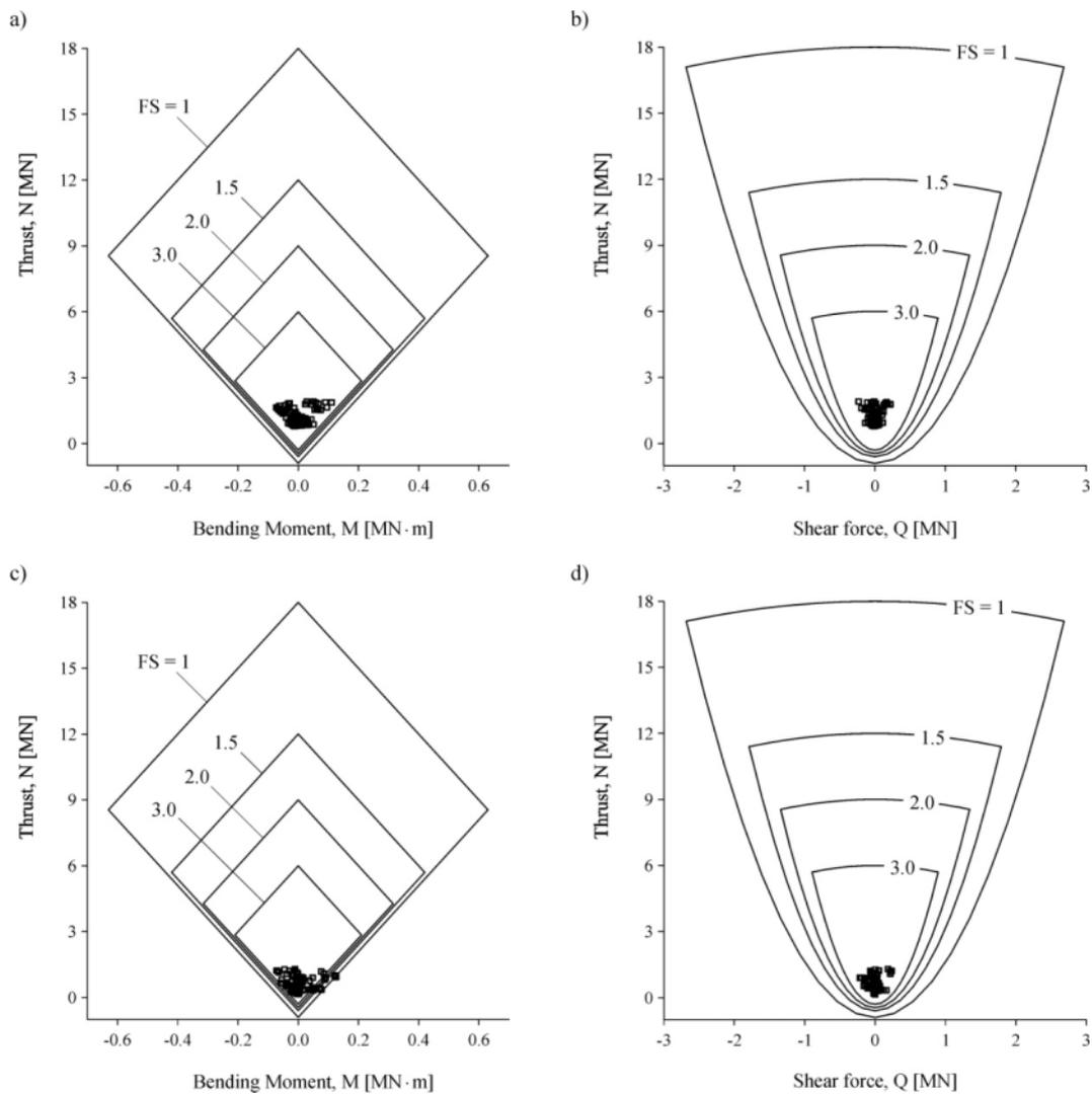
Figure 10. Capacity diagrams and support loading obtained from the Phase2 models corresponding to level 2,800 m (depth 200 m) considering a permanent concrete liner 0.5 m thick. Diagrams (a) and (b) correspond to the initial operation condition of the shaft at year 2013, while diagrams (c) and (d) correspond to the later operation condition at year 2031.
