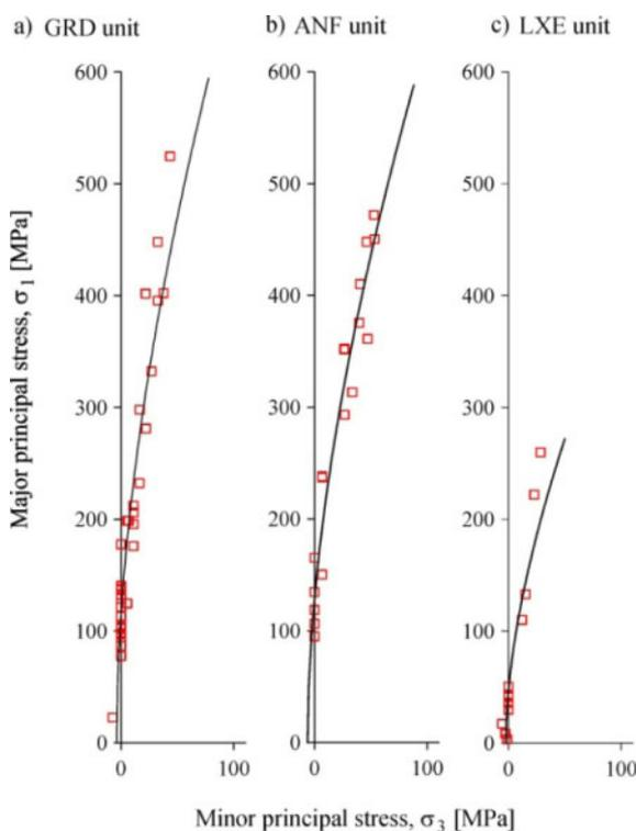
Figure 6. Shear strength failure envelopes for intact rock specimens for a) Granodiorite unit (GRD); b) Amphibolite unit (ANF); and c) Structurally Lixivated unit (LXE) as obtained from unconfined and triaxial compression testing.
