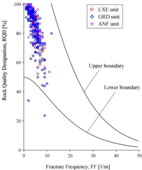
Figure 5. Relationship between Rock Quality Designation (RQD) and Fracture Frequency (FF) values for borehole CHDD8184.
