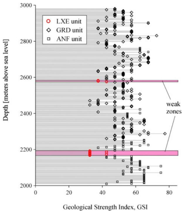
Figure 4. Distribution of the Geological Strength Index (GSI) as a function of depth, as interpreted from borehole CHDD8184 which coincides approximately with the axis of shaft PN-1.
