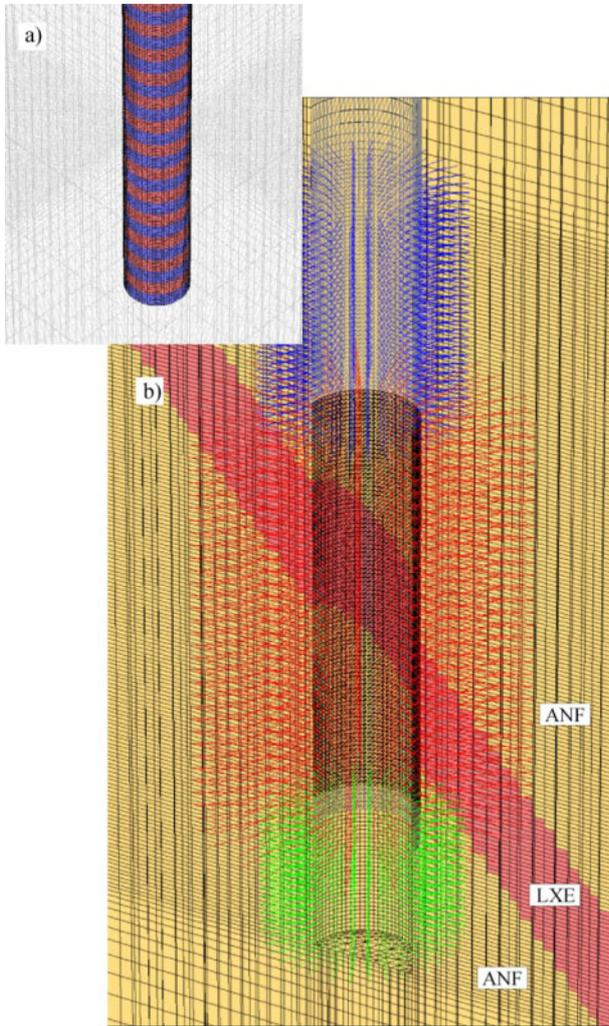
Figure 11. Three-dimensional numerical model of the advance of the shaft excavation through the Structurally Lixivated unit (LXE) at an approximate depth of 800 meters. The inset in the figure shows the 3 m advance intervals considered for the excavation of the shaft. The model, which incorporates temporary and permanent support, was constructed using the finite difference code FLAC3D – see Itasca (2007).
