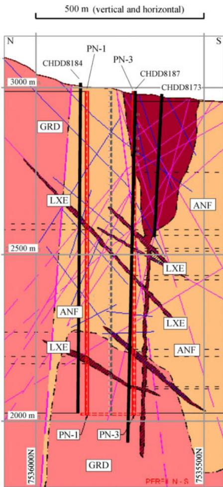
Figure 2. Vertical profile (with orientation North-South) containing the axis of shaft PN-1, indicating existing geotechnical units as interpreted from available geotechnical information.
