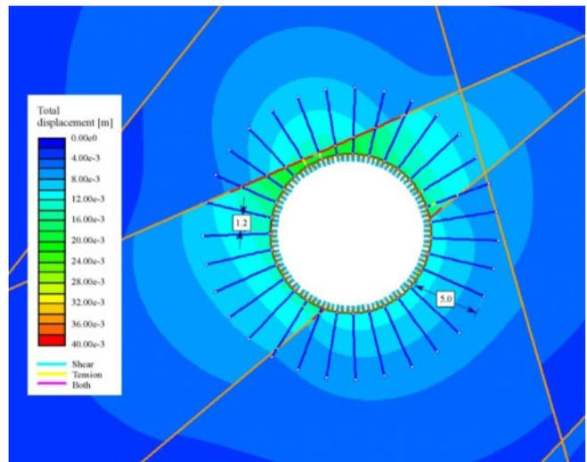
Figure 9. Resulting contours of displacements from a Phase2 model for level 2,500 m (depth 500 m), considering a combination of rock bolts 5 m long, spaced 1.2 meters in the circumferential direction, and 1.0 meter in the shaft axial direction, and with a permanent concrete liner of thickness 0.5 m.
