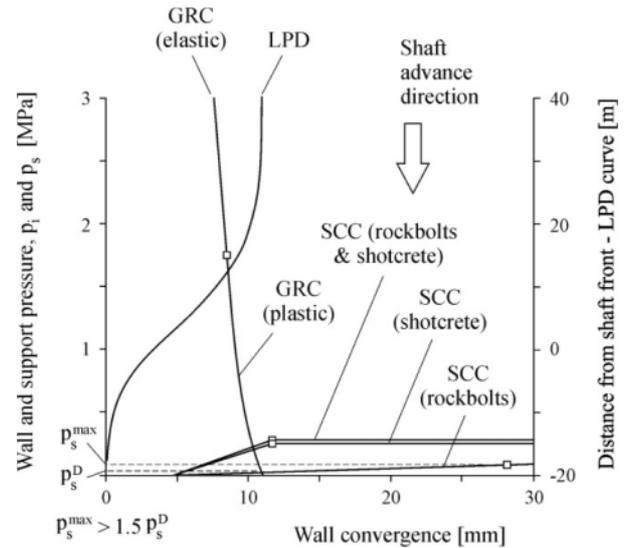
Figure 7. Application of the convergence-confinement method for shaft section PN-1 in the Granodiorite unit (GRD). The diagram represents the Longitudinal Displacement Profile (LDP), the Ground Reaction Curve (GRC) and different Support Characteristic Curves (SCC) considered – see Carranza-Torres & Fairhurst (2000) for equations used and construction of the diagram.
